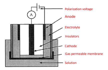
The sensor is composed of main components such as cathode, anode, electrolyte and semi-permeable membrane. Under the action of DC polarization voltage, oxygen dissolved in water goes through the semi-permeable membrane to the cathode for reduction reaction: O2 + 2H2O + 4e = 4OH
